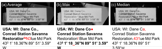
Fig. 2. OCR results for three different combining kernels (a) Average, (b) Max, and (c) Median.
