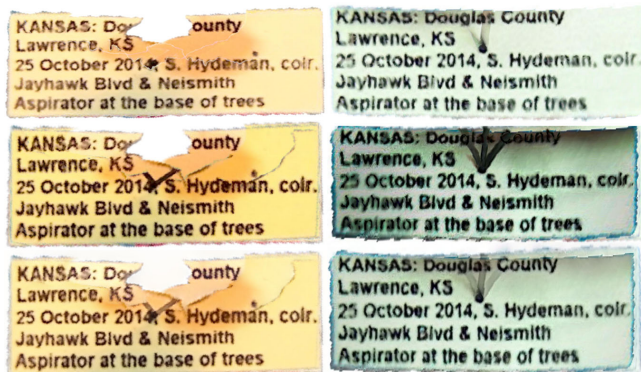
Figure 10. Two results of label composition using 3 views (left column are from top row of Fig. 1, right column are results from bottom row). Composition using the maximum value (top row) at each pixel removes the pin from the final composite image. Composition using the minimum value at each pixel (middle row) shows the accuracy of our non-linear text alignment process. For comparison we also performed composition using exposure fusion [26] (bottom row). A gap is seen in the composite image in the first column due to occlusion in all 3 views.
