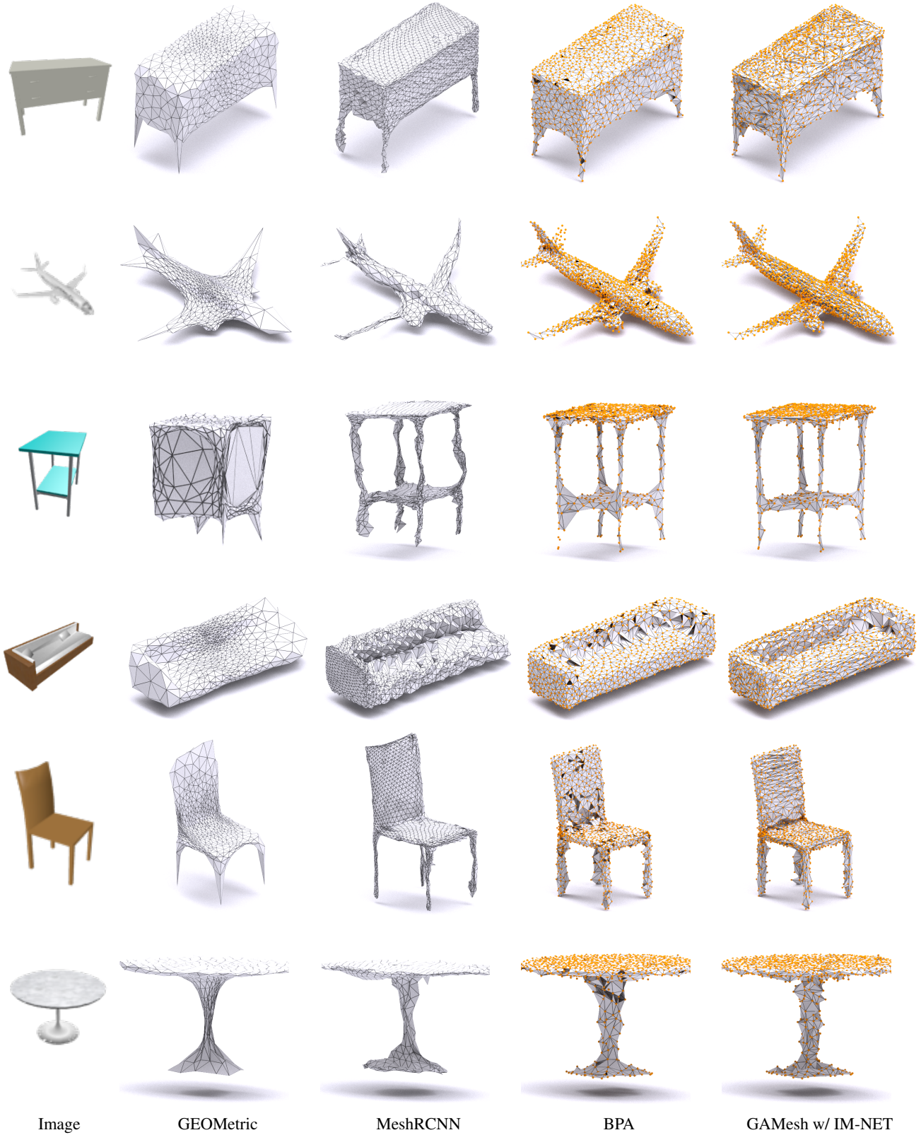
Figure 7: Single View Reconstruction. Qualitative comparison of ShapeNet testset meshes from various SVR approaches. Using meshes from IM-NET as priors, GAMesh reconstructs accurate surfaces for the output points (orange) of PSG + .
